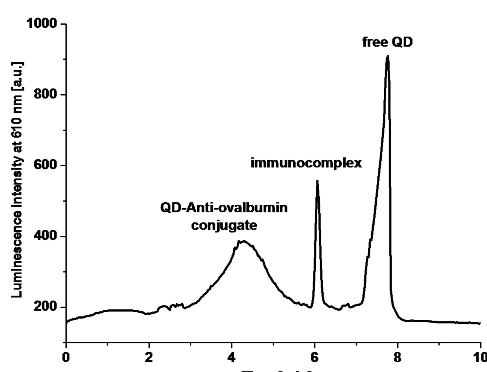
Separation conditions: fused silica capillary 15/25 cm, separation voltage 6 kV, injection time 15 s, separation buffer 100 mM TRIS/TAPS
