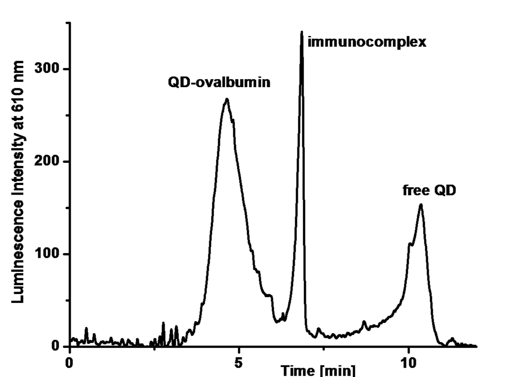
Separation conditions: fused silica capillary 15/25 cm, separation voltage 6 kV, injection time 6 s, separation buffer 100 mM TRIS/TAPS
