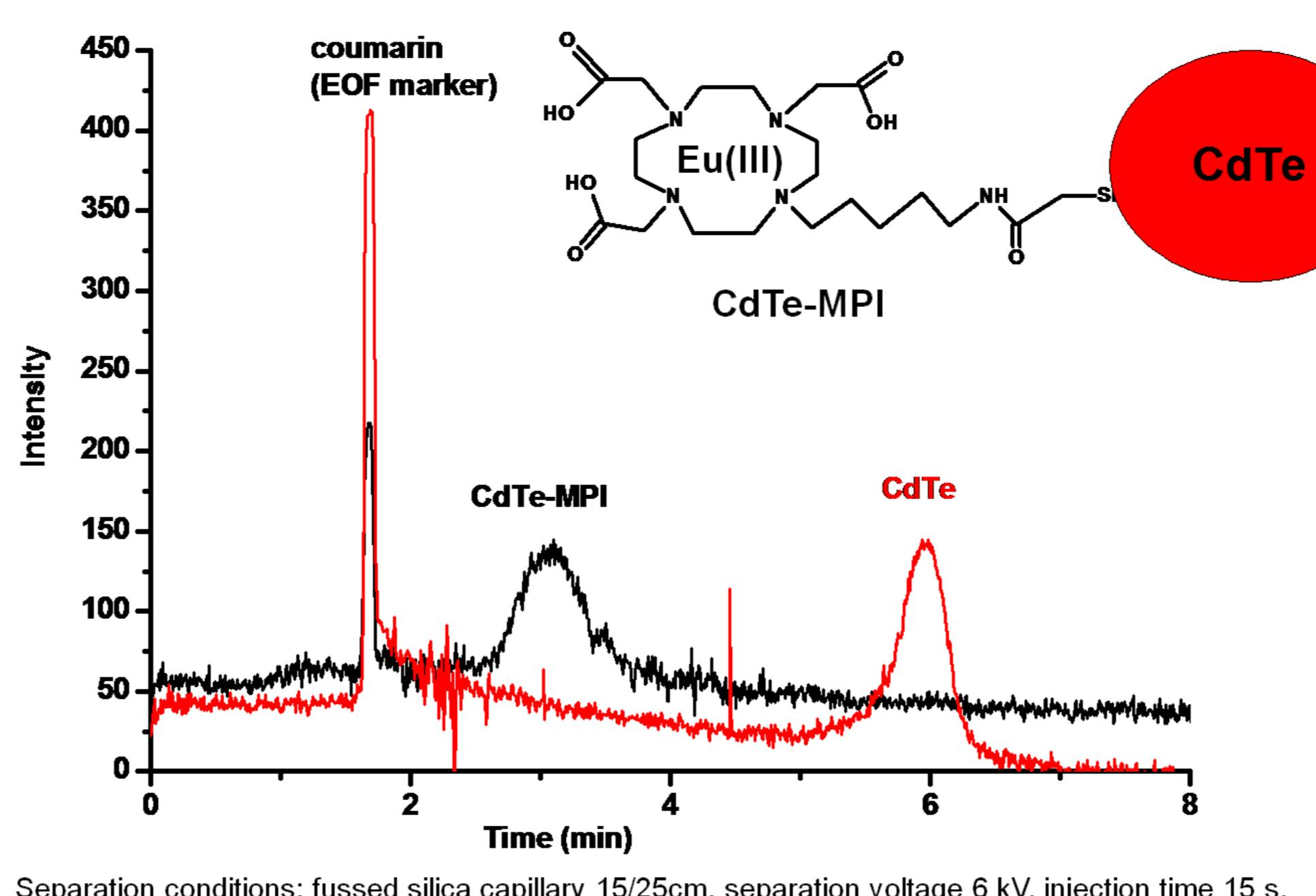
Separation conditions: fused silica capillary 15/25 cm, separation voltage 6 kV, injection time 15 s, separation buffer 100 mM TRIS/TAPS, pH = 8.3
