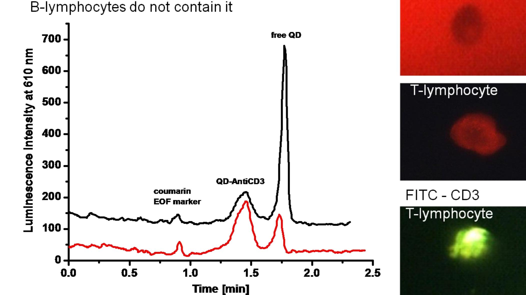
Separation conditions: fused silica capillary 12/20 cm, separation voltage 6 kV, injection time 15 s, separation buffer 50 mM CAPS, pH = 11.2
