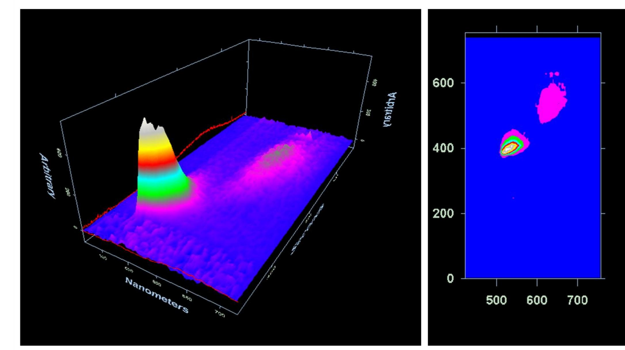
PVA coated capillary 20/30 cm, i.d. 75 mm, separation buffer 3% LPA 10 MDa in 50 mM TRIS/TAPS buffer, pH = 9, QD 2.8 and 3.7 nm (525 and 610 nm 1:1), injection time 10 s, separation voltage 3 kV
